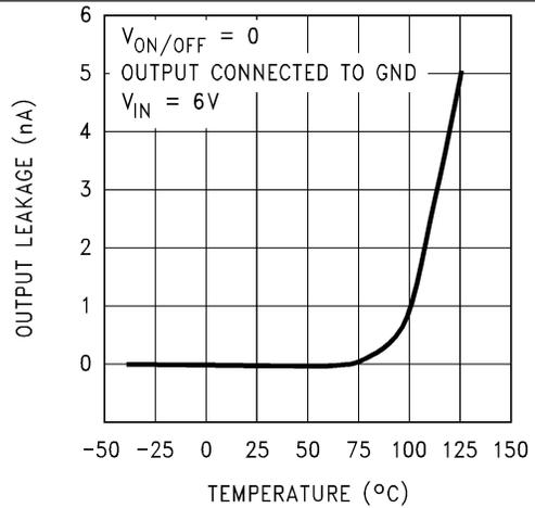
Figure 26. Input to Output Leakage vs Temperature
