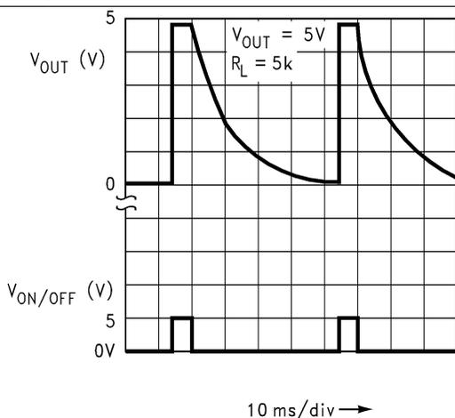
Figure 29. Turn-Off Waveform
