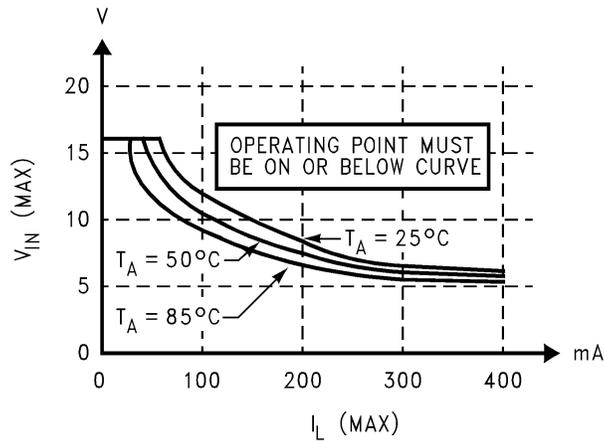
Figure 37. Safe Operation Boundary Curves for Figure 36
