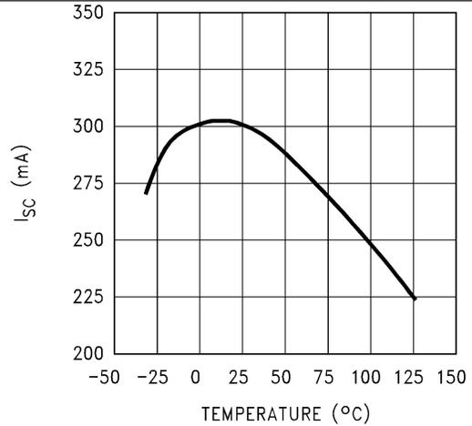
Figure 20. Instantaneous Short Circuit Current vs Temperature
