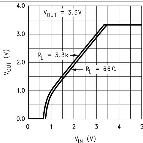
Figure 5. Dropout Characteristics
