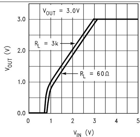
Figure 6. Dropout Characteristics
