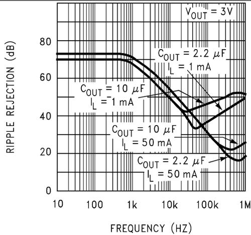
Figure 25. Ripple Rejection
