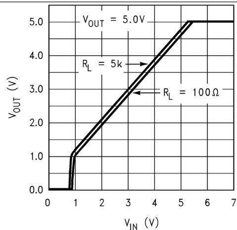
Figure 4. Dropout Characteristics
