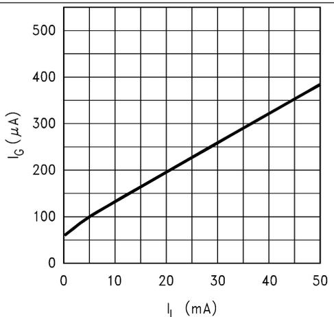
**Figure 10. Ground Pin Current vs Load Current**
